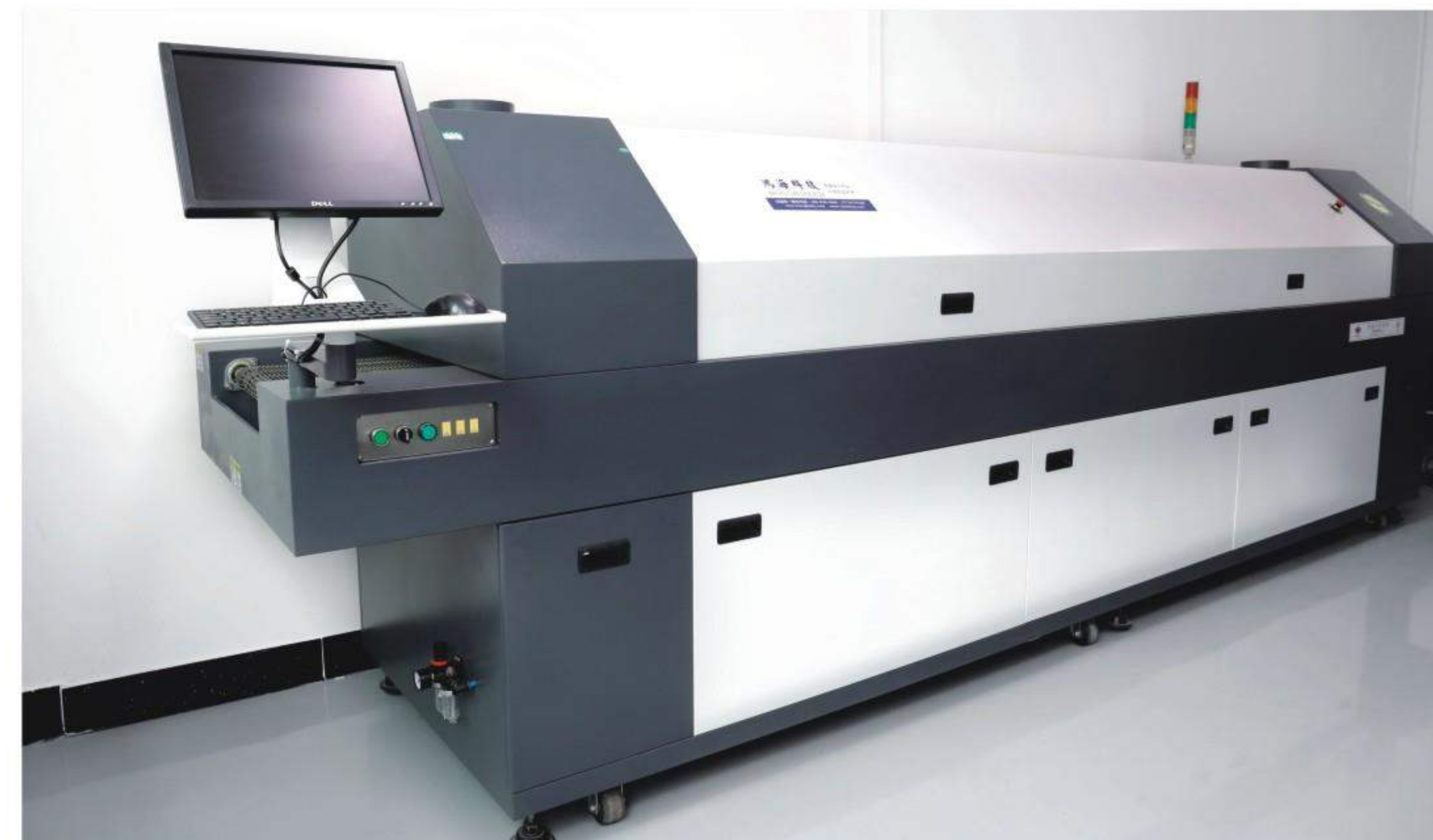
▲ 八温区全自动回流焊 Fully automatic reflow soldering with eight temperature zones
